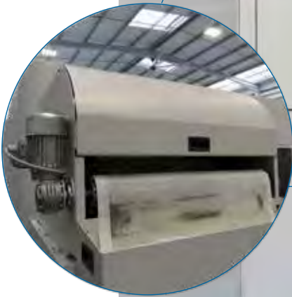
PAPER FILTRATION SYSTEM
