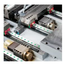
X/Y/Z/B Axes Roller Guideways provides rigidity and smooth axial movement for excellent machining and repeatability accuracy.
