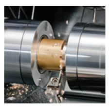
Spindle No. 2 is on the B-Axis and is servo motor driven for thrust and feedrate to help provide high precision movement and easy set-up. This feature alone can save up to 20% in operating efficiency over conventional designs.
