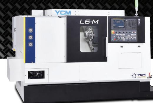
Mid range 2 axes machine (X/Z axis, live tooling and tailstock) for middle to upper range components.
